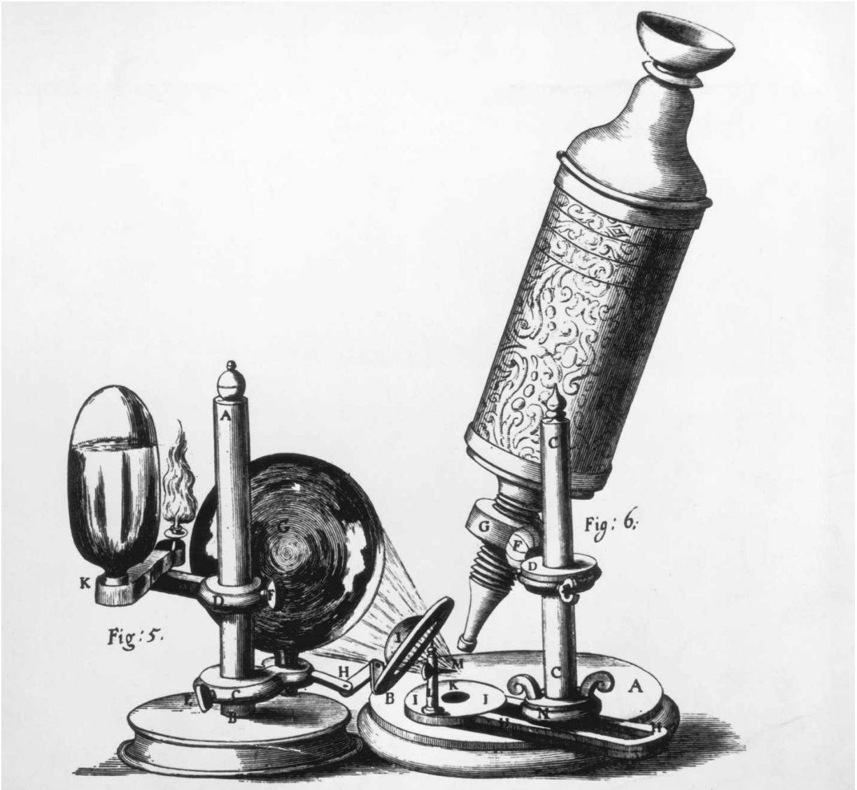
An early microscope designed by Robert Hooke, 1665
